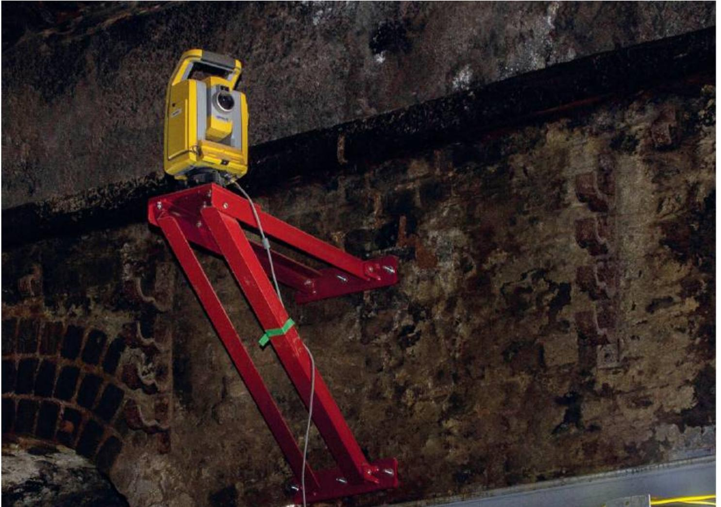
One of the five monitoring total stations in position in the tunnel.
